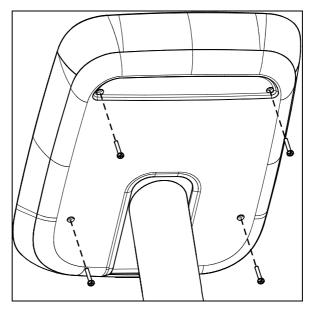
Figure 19: Reattaching rear cover screws
